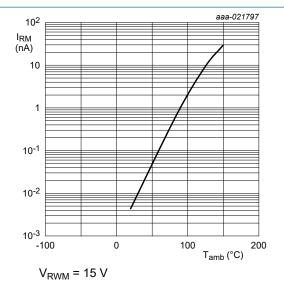
Fig. 7. Relative variation of reverse leakage current as a function of ambient temperature; typical
