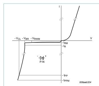
Fig. 4. V-I characteristics for a unidirectional TVS protection diode
