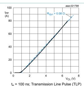
Fig. 9. Negative clamping voltage (TLP); typical values
