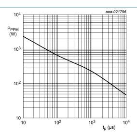
Fig. 5. Rated peak pulse power as a funtion of square pulse duration; typical values
