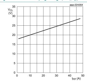
Fig. 10. Positive clamping voltage (8/20 μs pulse); typical values
