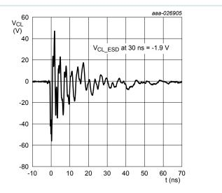
Fig. 14. Clamped -8 kV pulse waveform (IEC 61000-4-2 network)
