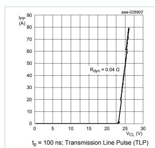
Fig. 10. Dynamic resistance with positive clamping voltage; typical values
