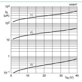
(1) T<sub>amb</sub> = 125 °C (2) T<sub>amb</sub> = 85 °C (3) T<sub>amb</sub> = 25 °C
