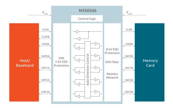
NXS0506 comes with auto-enable feature. If the supply voltage at Memory card side ( $V_{\rm CCB}$ ) rises above 1.5 V, the level translator logic is enabled automatically. As soon as  $V_{\rm CCB}$  drops below 0.65 V, the memory card side drivers and the level translator logic are disabled. The device features an auto correction control for all data channels except CLK.
