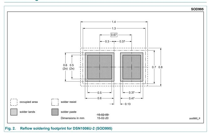
silicon, leadless ultra small package; 2 terminals; 0.325 mm pitch; 1 mm x 0.6 mm x 0.27 mm body
