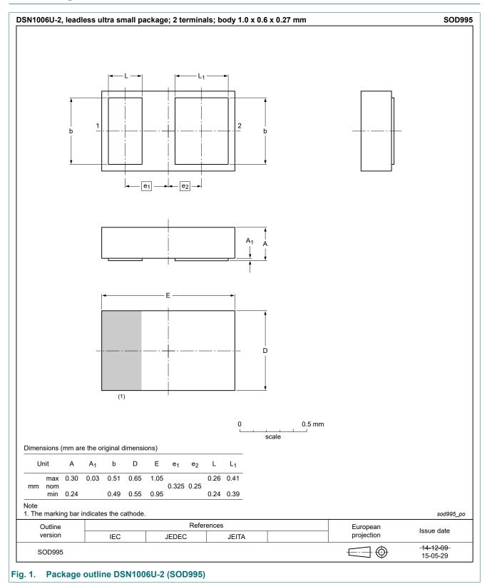
silicon, leadless ultra small package; 2 terminals; 0.325 mm pitch; 1 mm x 0.6 mm x 0.27 mm body
