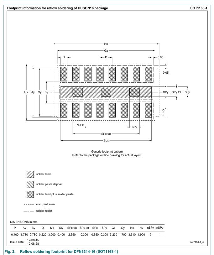
plastic, thermal enhanced ultra thin small outline package; 16 terminals; 0.4 mm pitch; 3.3 mm x 1.35 mm x 0.55 mm body
