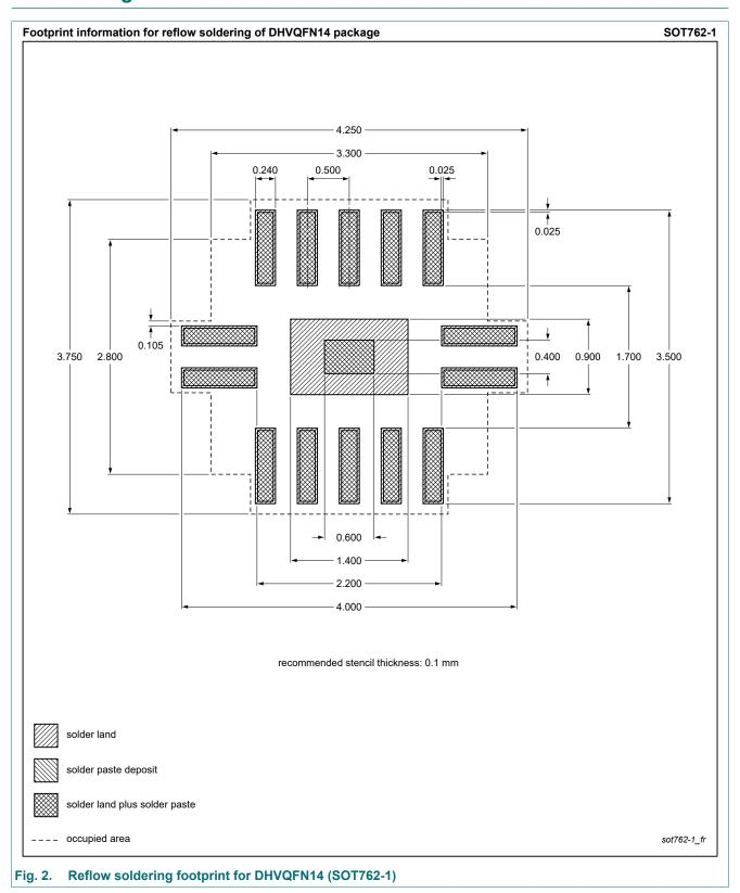
plastic, leadless dual in-line compatible thermal enhanced very thin quad flat package; 14 terminals; 0.5 mm pitch; 2.5 x 3 x 1 mm body
