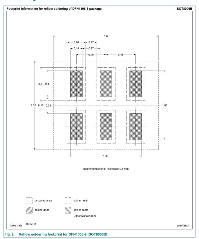
plastic, leadless extremely thin small package; 6 terminals; body 1.3 x 0.8 x 0.38 mm
