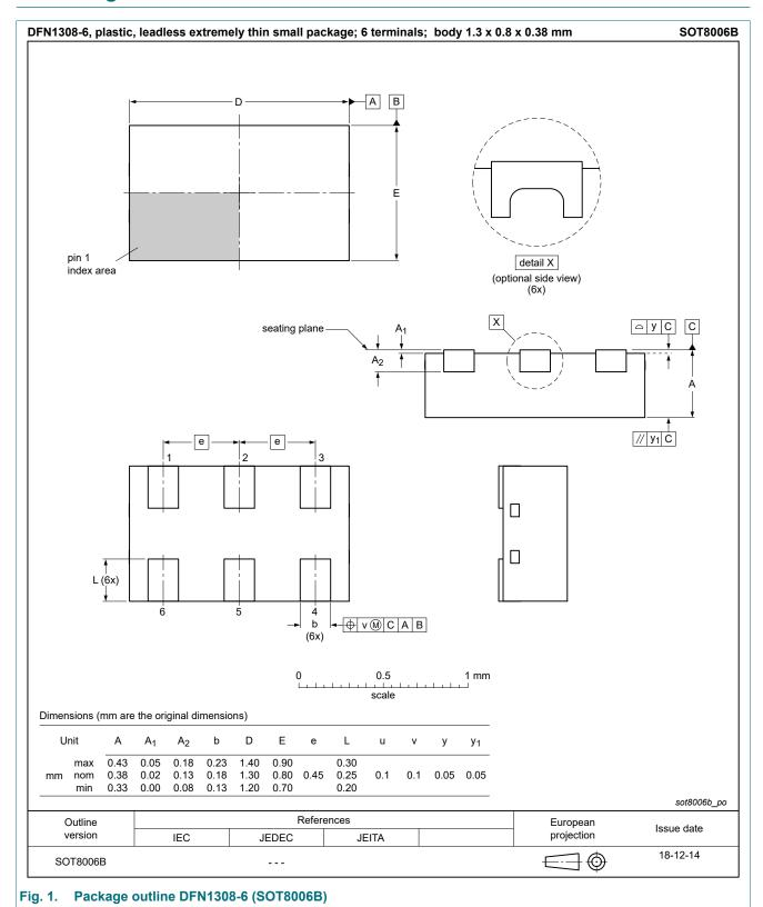
plastic, leadless extremely thin small package; 6 terminals; body 1.3 x 0.8 x 0.38 mm
